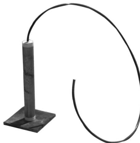
Fig. 1. The test arrangement of DMAZ sensitivity to standard detonator.
