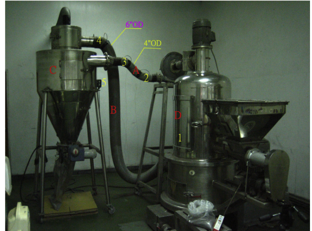
Fig. 2. Grinder. Electrostatic charge was measured at locations A, B, C, and D.
