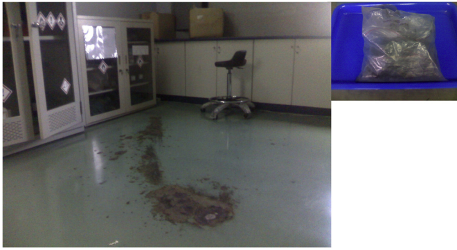
Fig. 1. Fire triggered by electrostatic charges when Ti-75 nanoparticles in polyethylene bag were taken from plastic plate.
