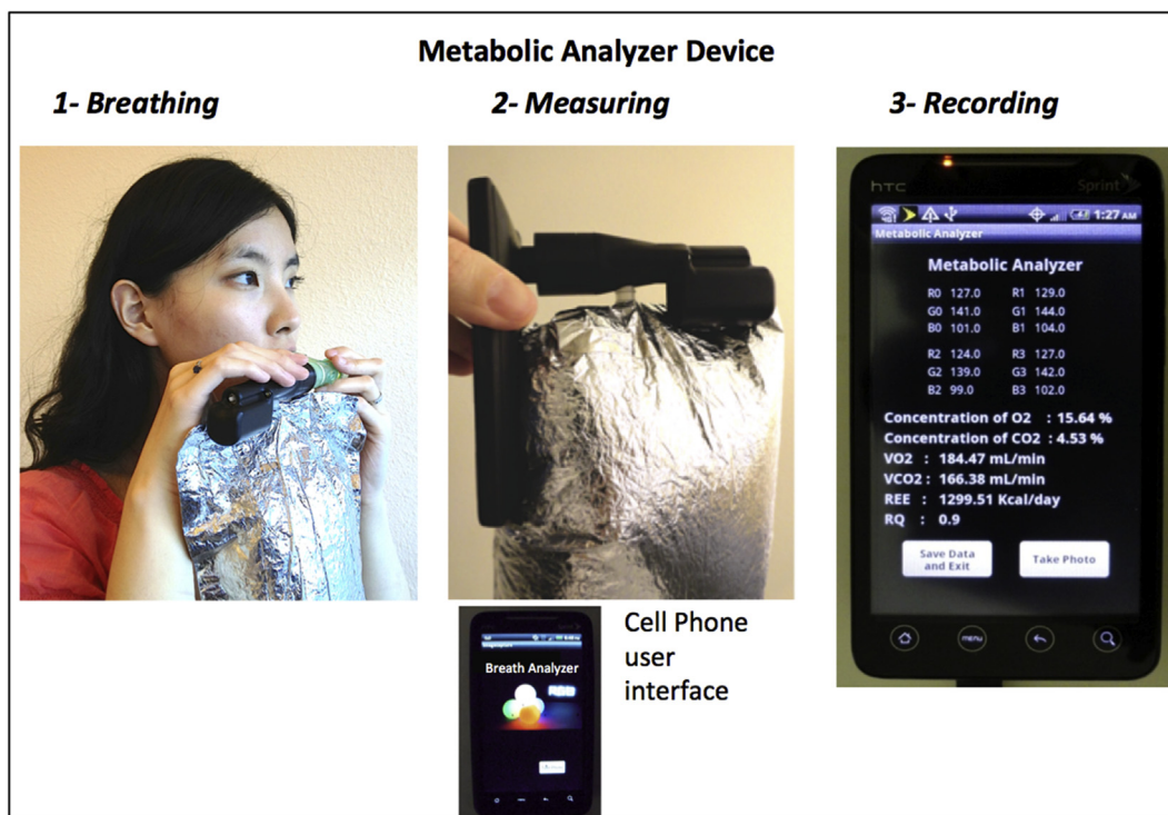
Fig. 1. Metabolic analyzer device. The device simultaneously detects the consumed oxygen and produced carbon dioxide, and the exhalation rate, from which energy expenditure is determined. It is paired to a cell-phone, which records the metabolic parameters, and track the personal metabolic history of users. Sequence of use: 1- Use of the sensor integrated mouthpiece to collect breath sample. 2- The sensor integrated mouthpiece is assembled to the cell-phone to analyze the sensor signal. 3- The user interface in the cell phone displays the results.
