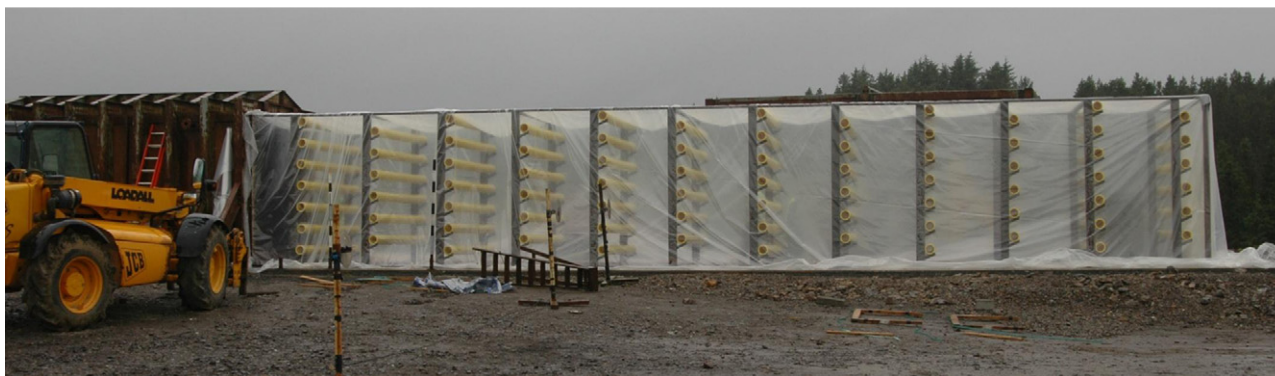
Fig. 1 – The test rig with congested region covered in polythene prior to gas filling.
