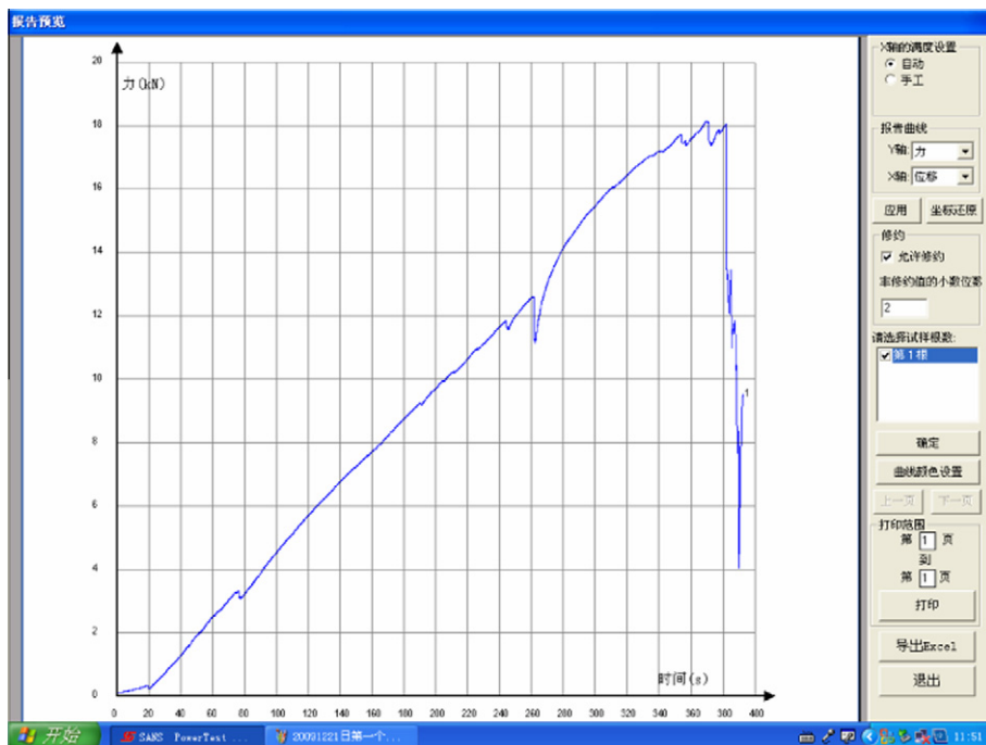
Fig. 2. The relationship between stress and loading time under uniaxial compression of Laohutai coal sample.
