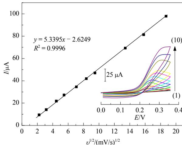
Fig. 2. Plot of  $I_{pa}$  versus  $v^{1/2}$  for the oxidation of ISPR by the PGRMMWCNTPE. The inset shows cyclic voltammograms for various scan rates of 5 (1), 10 (2), 20 (3), 30 (4), 50 (5), 70 (6), 90 (7), 180 (8), 250 (9), and 350 mV/s (10) in 0.1 mol/L PBS (pH 7.0).
