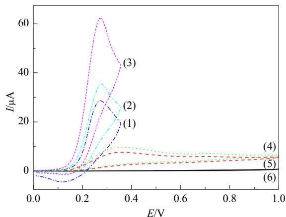
Fig. 3. Cyclic voltammograms of PBS at the PGRMMWCNTPE (1), 500  $\mu\text{mol/L}$  ISPR at the PGRCE (2), PGRMMWCNTPE (3), CNPE (4), and CPE (5), and PBS at the CNPE (6). Conditions: 0.1 mol/L PBS (pH 7.0) and scan rate 20 mV/s.
