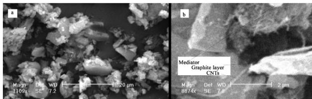
Fig. 1. SEM images of (a) the CPE and (b) the PGRMMWCNTPE.
