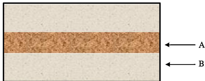
Fig. 1. Schematic diagram of the cross section of a channeled sandpack. (A) Coarse sand in the channel in the center of the holder. (B) Fine sand in the annulus.
