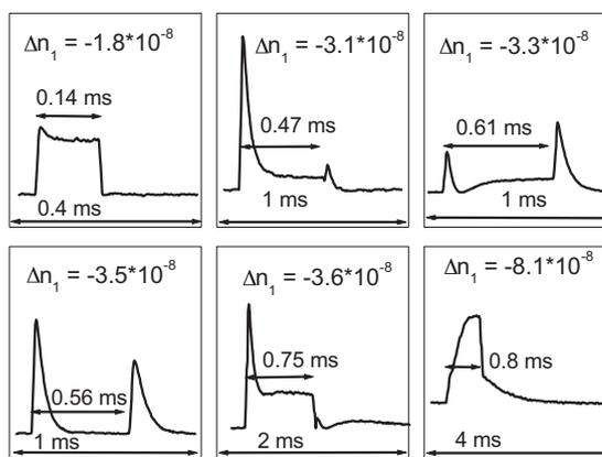
**Fig. 2.** EB signals from  $C_8F_{17}SO_3N(C_2H_5)_4$  at constant field  $E = 11.9 \times 10^4$  Vm $^{-1}$  at  $25^\circ C$  for increasing concentrations of (from top left to bottom right): 5, 8, 10, 12, 13 and 14 mM. Pulse lengths (0.14 ms to 0.8 ms) are indicated by arrows to show when the E-field was switched on and off, respectively.
