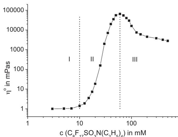
**Fig. 1.** Zero-shear viscosity of  $C_8F_{17}SO_3N(C_2H_5)_4$  aqueous solutions as a function of concentration at  $T = 25^\circ C$ .
