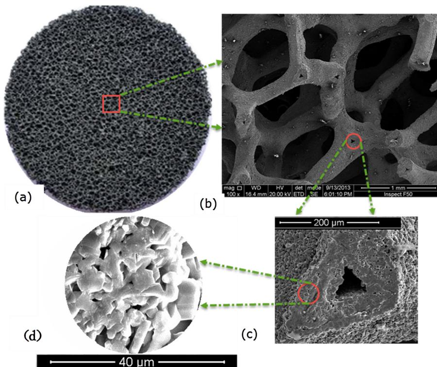
**Fig. 1.** Photograph of a section of SiC foam sample (a), scanning electron microscope photographs of the cell structure (b), triangular cross section of hollow skeleton (c), and micro-pores throughout the strut of foam skeleton (d).
