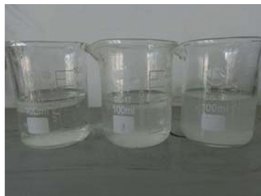
Fig. 2. Compatibility study between different alkalines with 0.04 wt% \text{CaCl}_2 solution (from left to right the alkaline are ethylenediamine, NaOH and \text{Na}_2\text{CO}_3 respectively, the alkaline concentration is 0.5 wt%).
