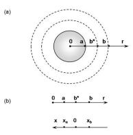
**Fig. 2.** (a) Scheme of a two-layer spherical cell model. (b) Scheme of transition from the old system of coordinates (r) to the new one (x).
