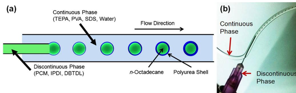
**Fig. 1.** (a) Schematic diagram of the fabrication of monodisperse PCM@polyurea microcapsules in a tubular microfluidic device and (b) photograph of O/W PCM droplets produced at the tubular junction. Emulsification and partial polycondensation occur in the flow stream at 35 °C.
