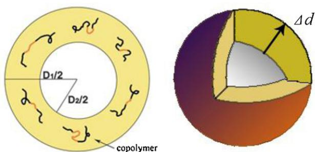
**Fig. 1.** Schematic diagram of polymer in the nanosphere, a cross-section view (left) and stereopicture (right).
