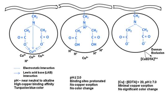
**Fig. 1.** Schematic illustration of interactions between copper and IDA functionality, at near neutral to alkaline pH, at pH  $\leq$  2.0 and in the presence of EDTA around neutral pH.
