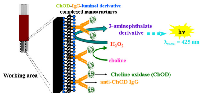
Scheme 3. Reagentless detection principle of choline oxidase activity by ECL reaction triggered directly in the sensing layer.
