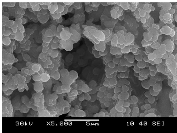
Fig. 2. SEM image of  $ZrO_2$  film assembled with BSA.
