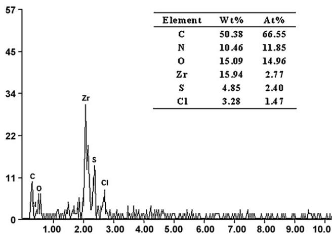
Fig. 3. EDS image of  $ZrO_2$  film assembled with BSA.
