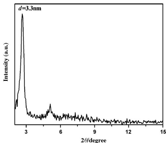
Fig. 1. XRD pattern of  $ZrO_2$  film assembled with BSA.
