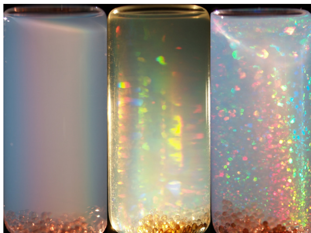
Fig. 2. Images of the sample vials for different compositions p and particle number densities n . Image size approx. 14 mm × 35 mm. (From left to right) Featureless fluid structure at p = 0.9 and n = 5.92 \pm 0.01\ \mu\text{m}^{-3} ; columnar wall based crystals at coexistence at p = 0.15 and n = 0.53 \pm 0.05\ \mu\text{m}^{-3} ; bulk nucleated crystals at coexistence at p = 0.9 and n = 0.59\ \mu\text{m}^{-3} and a polycrystalline sample at p = 0.15 and n = 1.24 \pm 0.12\ \mu\text{m}^{-3} .
