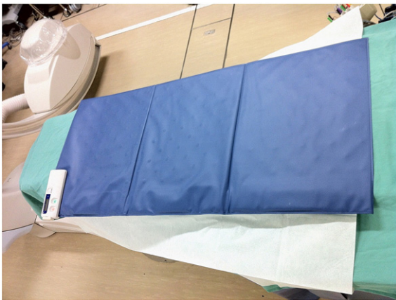
Fig. 1. SD-101 sleep recorder; a sheet shaped portable respiratory monitor which has 162 pressure sensors in its body to detect events of disordered breathing and changes in body position.
