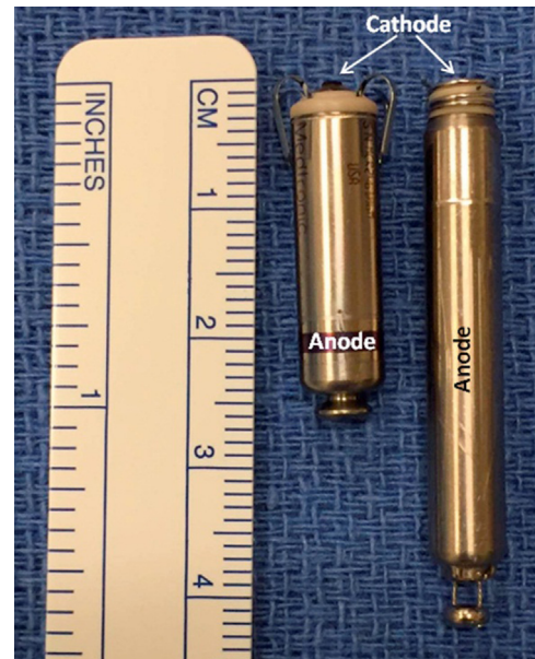
Fig. 1 – Leadless Pacemakers [14]. The Micra Transcatheter Pacing System (left) and Nanostim leadless cardiac pacemaker (right) are shown next to a ruler. The active fixation (cathode) tines can be seen. Both devices are retrievable by catheter attachment at the proximal (anode) end. (Color version of figure is available online.)
