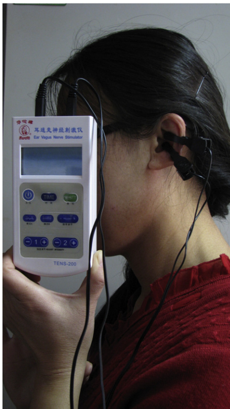
Fig. 1. The ta-VNS device, the stimulator clips, and the stimulation positions at the concha cavity and the concha cymba.
