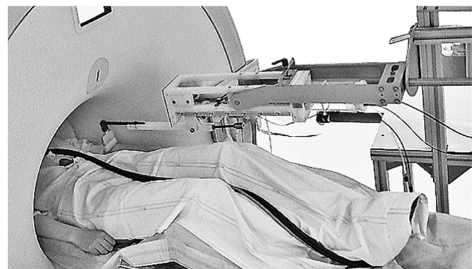
Fig. 1. Linear tactile stimulator for high-precision brush stroking of the left forearm.
