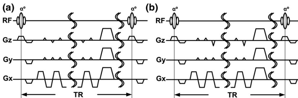
**Fig. 1.** The blipped-InI pulse sequences to achieve (a) FOV/2 and (b) FOV/3 in-plane shifts. In (a), the  $G_z$  blips change the polarity alternatively between read-outs but have the same magnitude of gradient moment. Such  $G_z$  blips can induce FOV/2 in-plane shift. In (b), the  $G_z$  blips have the repetitive “up-up-down” pattern across read-outs. The downward  $G_z$  blips have twice the gradient moment of the upward  $G_z$  blips. Such  $G_z$  blips can introduce FOV/3 in-plane shift.
