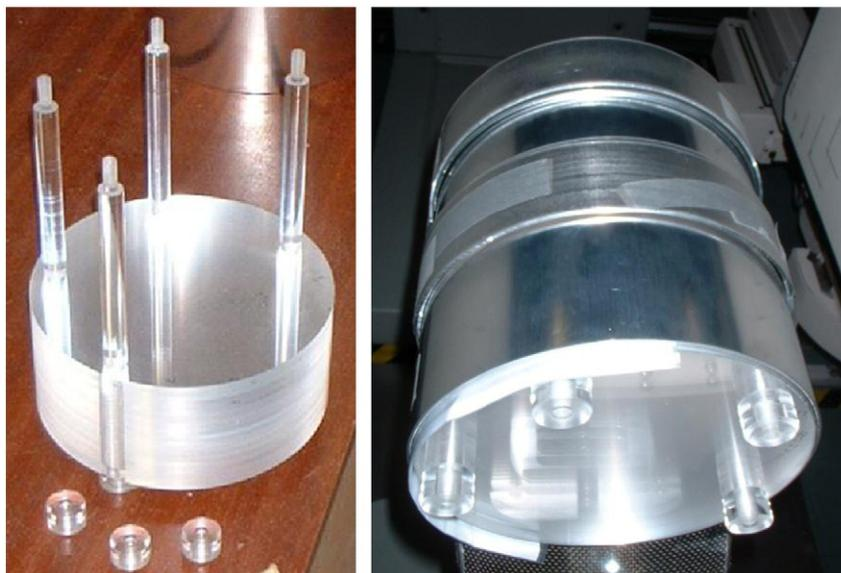
Fig. 1. Partially disassembled (left) and fully assembled (right) views of the sandwich rCBF phantom.
