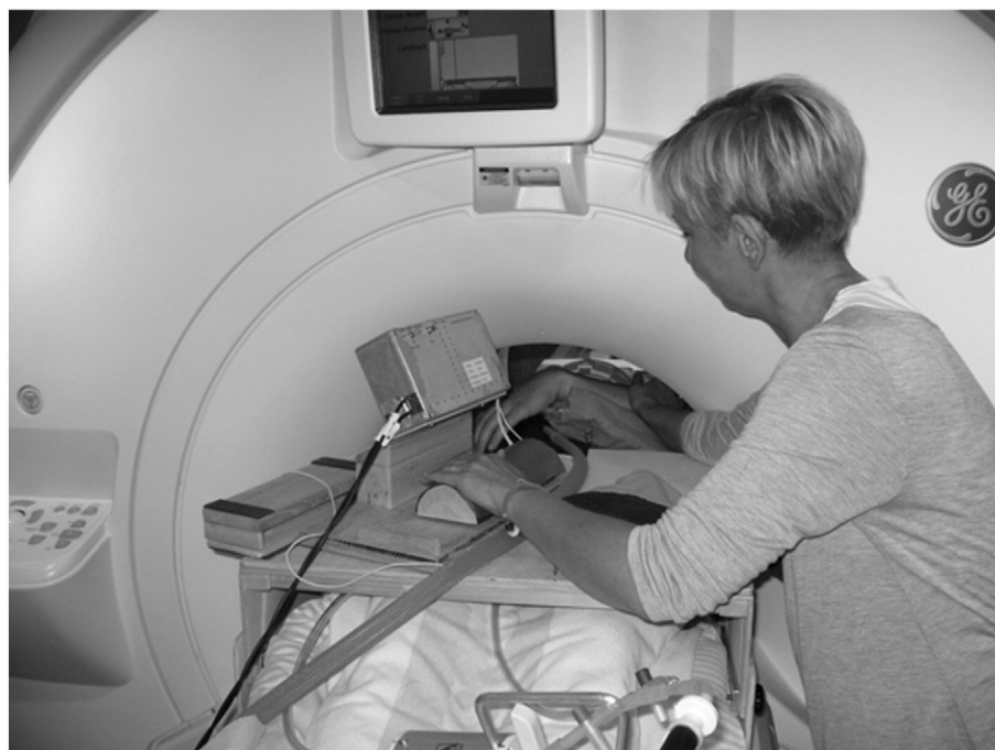
Fig. 1. Touch conditions. A touch device in the scanner room indicated the different touch conditions, the correct force (2.5 N) and the correct velocity (1–5 cm/s). The force of the mirror movement applied on the dummy arm was measured by force transducers and sampled in a computer.
