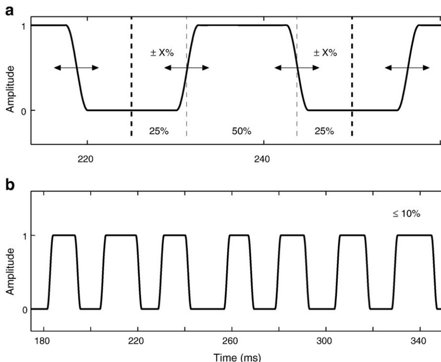
**Fig. 1.** Time waveforms of the square-wave modulator. (a) Irregular square waves are generated by jittering the onset and offset times within each period. (b) Example of the square-wave modulators with a 10% degree of maximum jitter. The modulator is convolved with a 5-ms Hanning window.
