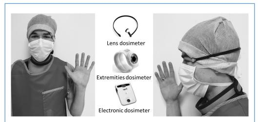
Figure 1. Representation of the different dosimeters used for the study and a diagram representing an operator wearing dosimeters and the proper protective equipment.
