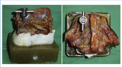
Figure 1. Anterior vertebral bodies were mounted with polymethylmethacrylate and polyester resins in the potting fixtures of a material testing machine.
