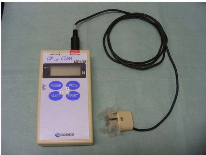
Fig. 1. Lip Closure Strength (force) Indicator (Lip De Cum ® ) with a Lip holder (Ducklings ® ).
