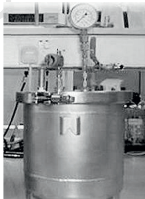
Fig. 1 – Schematic of treatment and assay regimes (A). Image of hyperbaric culture chamber used in HBO exposures (B).
