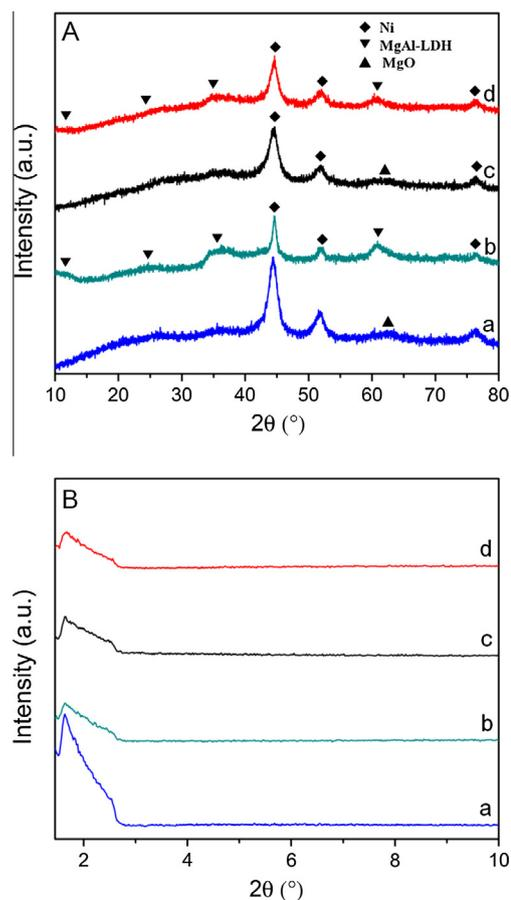
**Fig. 1.** Wide-angle (A) and small-angle (B) XRD patterns of the prepared core-shell nanocomposites. Ni@mSiO<sub>2</sub>@LDO (a), Ni@mSiO<sub>2</sub>@LDH (b), Ni@mSiO<sub>2</sub>@LDO-C (c), and Ni@mSiO<sub>2</sub>@LDH-R (d).
