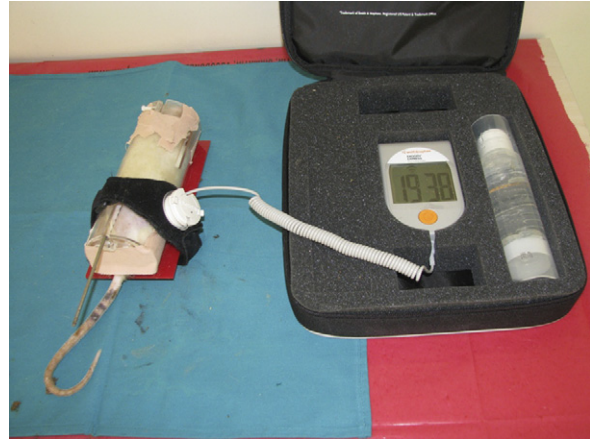
Fig. 2. The ultrasound transducer was only attached to the lateral surface of the right femurs of the group A animals.
