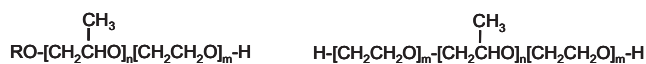
Fig. 1. Chemical structure of polyalkylene glycols (PAGs) (left) and co-polymer of polyethylene oxide and polypropylene oxide (Pluronic) (right).
