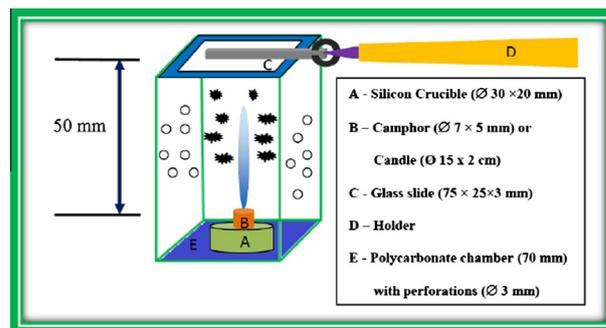
Fig. 1. Schematics for collection of soot particles of combustion of camphor and candle.
