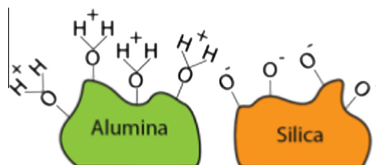
Fig. 1. Schematics of a physical mixture of alumina and silica immersed in an aqueous solution where \text{PZC}_{\text{silica}} < \text{pH} < \text{PZC}_{\text{alumina}} .
