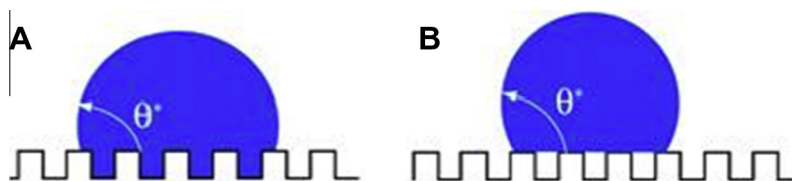
Fig. 1. A schematic illustration of the formation of composite interfaces with a droplet in the Wenzel (A) and Cassie–Baxter (B) state.
