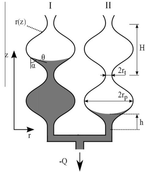
Fig. 1. Definition sketch of two hydraulically connected sinusoidal capillaries with pore throat radius  $r_t$  and pore body radius  $r_p$ . The distance between two throats (constrictions)  $H$  defines pore length. The inclination of the wall is given by  $\alpha$ , and the contact angle is indicated by  $\theta$ . Height of the interface is marked with  $h$ . Liquid is withdrawn with constant flow  $Q$ .
