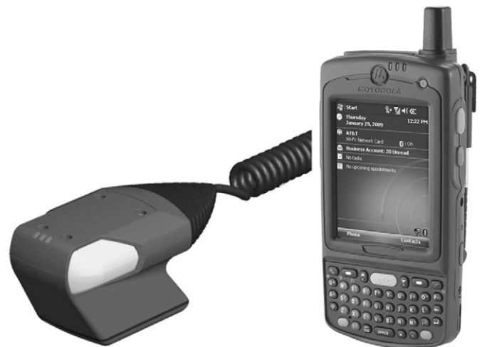
Fig. 3. The Pneumoscan device is shown. The MIR – antenna (left) is connected to a Motorola MC75 enterprise digital assistant (right). The results obtained from the scan are shown in real time.
