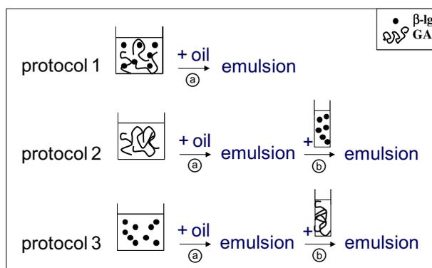
**Fig. 1.** Schematic depiction of the three protocols for emulsion preparation with  $\beta$ -lg and GA at 2:1 and 1:2  $\beta$ -lg:GA ratios. (a) Rotor-stator and high pressure homogenizers. (b) Hand reversal shaking.
