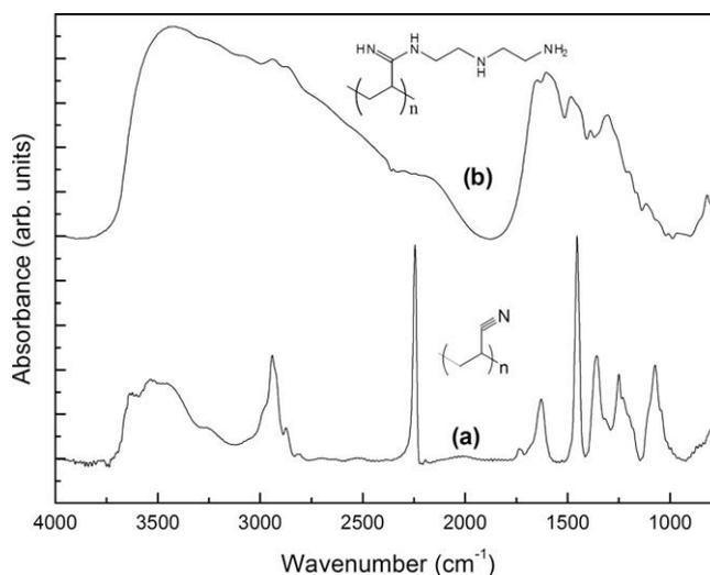
Fig. 1. FT-IR spectra of (a) raw PAN and (b) PADD.
