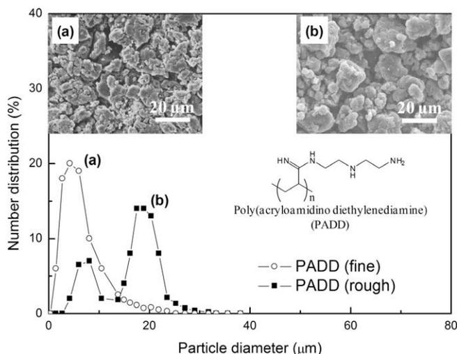
Fig. 2. FE-SEM images and the size distribution of (a) PADD (fine) and (b) PADD (rough).
