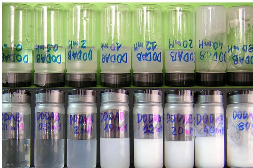
**Fig. 1.** Phase behavior of DODAB dispersions over the concentration range 0.1–80 mM at room temperature. The numbers on the photos express the concentration. Lower photos illustrate the transformation from turbid dispersions into milky ones with the concentration. Upper photos show the viscoelasticity of the dispersions.
