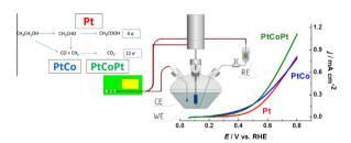
Structured PtCo nanoparticle catalysts were prepared with ALD method and their activity for ethanol oxidation was studied with electrochemical methods. PtCoPt-cycled catalyst showed significant activity and durability at elevated temperatures.
