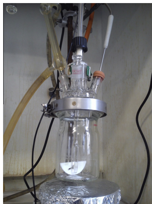
Fig. 1. Suspension polymerization reactor used in this study.
