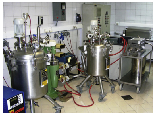
Fig. 1. Pilot scale plasma fractionation.
