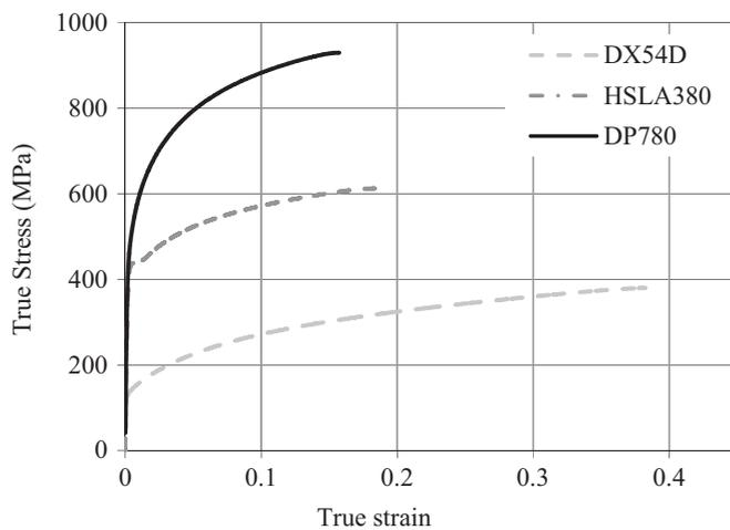
Fig. 1. Tensile test curves of the three materials studied in rolling direction.
