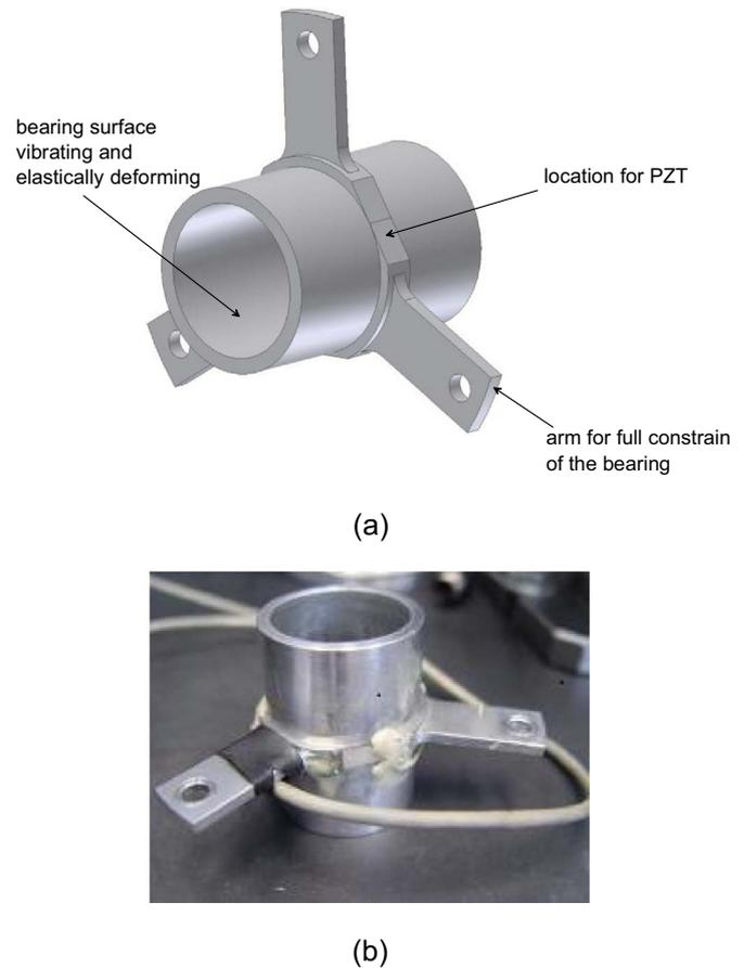
Fig. 1. (a) Solid modelling image of the bearing; (b) photograph of the bearing with PZTs.
