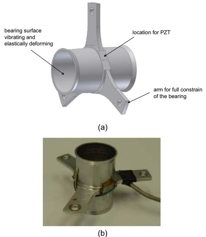
Fig. 2. (a) Solid modelling image of the bearing; (b) photograph of the bearing with PZTs.
