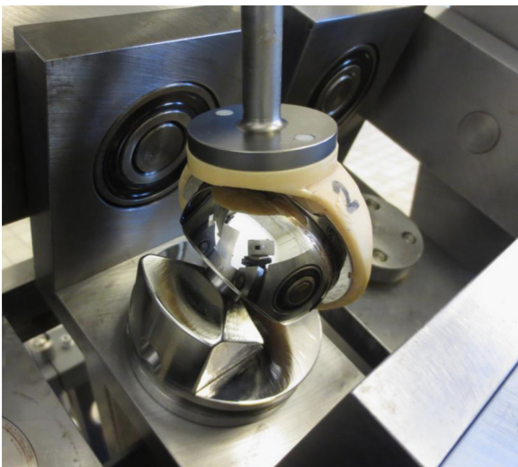
Fig. 1. Close-up of test station no. 2 of HUT-4 hip joint simulator showing 50 mm diameter Metasul MoM hip installed, without lubricant chamber. Gait of right hip is simulated. Durom acetabular cup is cemented to a position of 70^\circ inclination ( 66^\circ abduction, 32^\circ anteversion). At this moment, i.e., maximum extension (outer cradle) and neutral abduction–adduction (inner cradle) of the femoral head, and maximum load of the second (toe-off) load peak (vertical loading bar above the joint), high friction almost dislocates the joint as the motion is momentarily purely abduction of head. Hence, 70^\circ proved to be close to the highest possible inclination angle that could be run with.
