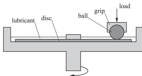
Fig. 1. Schematic of the ball-on-disc tribometer.
