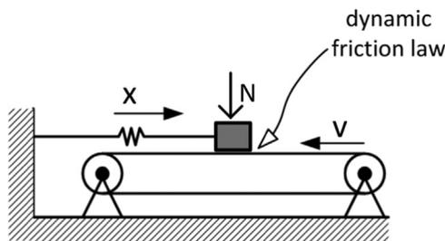
Fig. 1. Oscillator with dynamic friction law.
