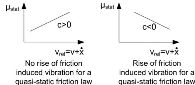
Fig. 2. Velocity-dependency of a quasi-static friction law and expected stability or instability of the system.
