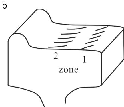
Fig. 1. Surface cracks of wheel tread, (a) surface oblique cracks; (b) definition of zones of cracks on the wheel treads.
