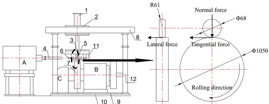
Fig. 2. JD-1 wheel/rail simulation facility and scheme size of simulating wheel and rail rollers. 1. Normal loading cylinder; 2. Loading carriage; 3. Spindle and yoke; 4. Universal shaft; 5. Wheel roller; 6. Wheel shaft; 7. Rail roller; 8. Lateral loading cylinder; 9. Turning plate; 10. Base plate; 11. Magnetic powder brake; 12. Speed measuring motor; A, B. ZQDR-204 DC motor; C. Gear box.
