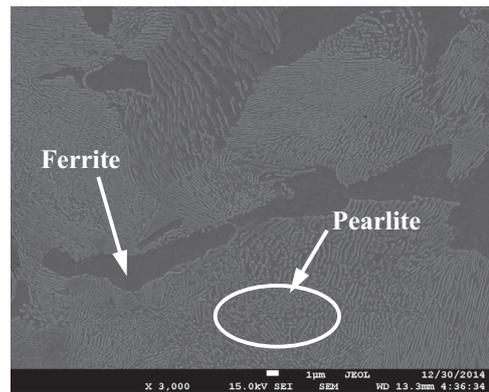
Fig. 3. Microstructure of wheel material.
