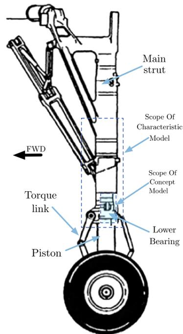
Fig. 1. Main landing gear (MLG) [1].
